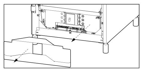
Route the dedicated PE battery cable through the dedicated opening in the bottom of the classic battery cabinets and connect them to the PE terminal.
